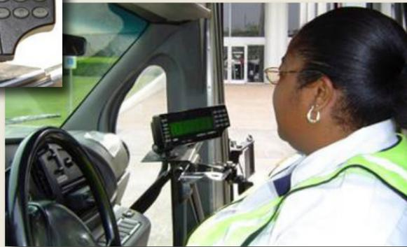
Mobile Data Computer (inset) installed on a bus
