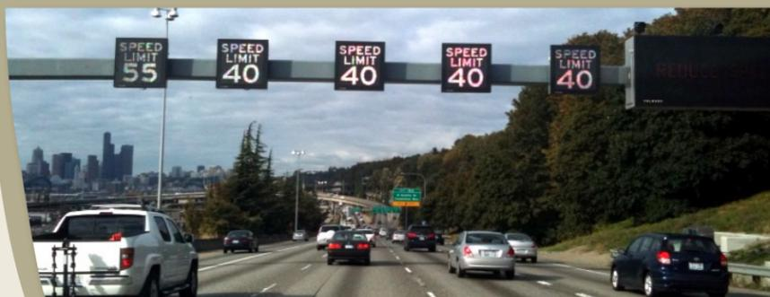
How do variable speed signs work? Traffic sensors or cameras along the roadway collect data on traffic speeds, identifying events such as temporary bottlenecks or accidents. Central computers reduce speeds in some or all lanes behind an event to gradually minimize the approaching flow of traffic.
