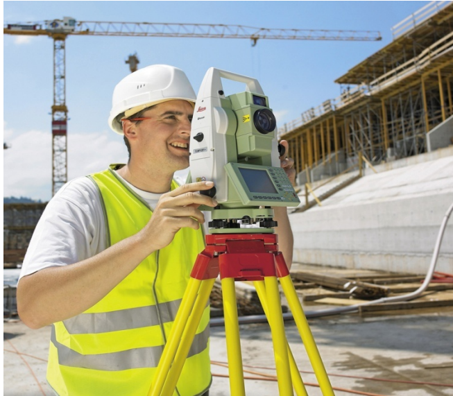
Figure A-2. Total Station Tool
