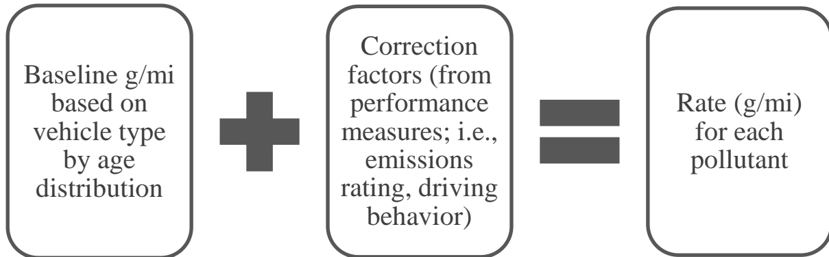
Figure 15: Basic method of determining pollutant rates.
