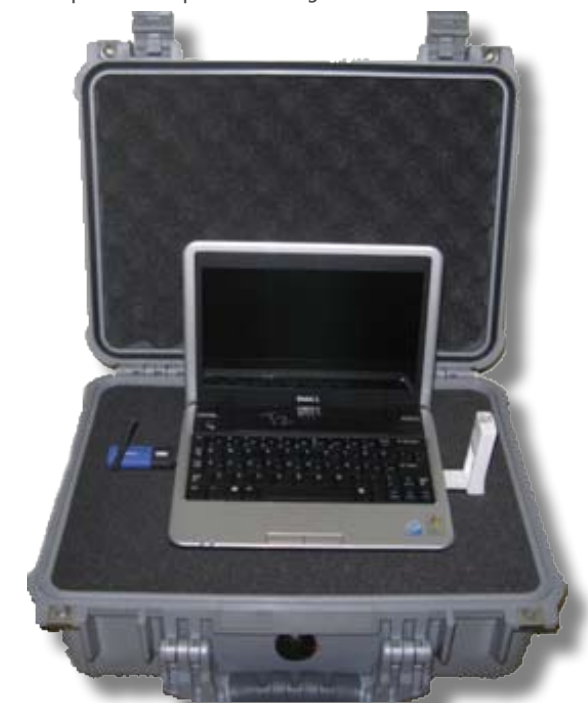
This roadside equipment prototype was deployed in Dayton, Ohio to detect MAC addresses from Bluetooth devices in vehicles as they passed by.
